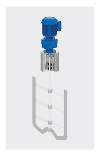
Anchor impellers are used specially for highly viscous flow, typical of polymer reactions. The viscosity is normally in the range 5,000-100,000 cp. Since this range of viscosity describe highly viscous flows, the reactions for anchor agitated systems are normally carried out under laminar flow. This work presents a detailed computational fluid dynamics (CFD) approach to study the behaviour of stirred vessels using anchor impellers.
