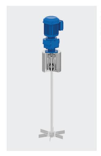
The Rushton turbine is a radial flow impeller used for many mixing applications. The design is based on a flat disk with vertical, flat blades vertically mounted. Rushton turbines are very effective for gas dispersion. To some extent, this can be attributed to the way the rotating disc on the turbine captures gas released below the impeller and channels it into the regions of high turbulence near the blades.
